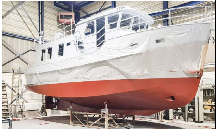
Painting of vessel hull in the shipyard workshop / shelter.
