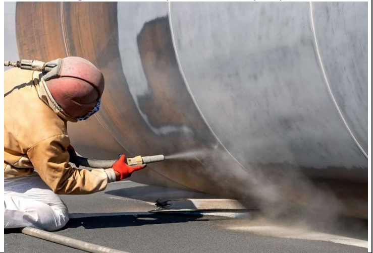
Hull repairs, Water blasting of vessel dry docked on slipway
